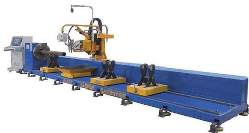
JINFENG® is the professional China manufacturer and supplier of Pipe cutting machine with chuck with affordable price. The Pipe cutting machine with chuck are high performance plasma and oxy flame 3D cutting machine to execute the plasma cutting or oxy flame cutting on round pipe or tube.
